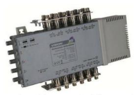
smaller to medium cascaded networks. These mains-powered multiswitches can be used to power up to six line powered multiswitches and an LNB. EV5-xxxM will power a Quattro LNB via the horizontal and vertical inputs at up to 650mA max. Power is provided from the built-in switch-mode power supply.
